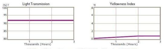
1/8" Nominal Thickness. Xenon arc per ASTM D 2565, Type B. Tested per ASTM D 1003.
